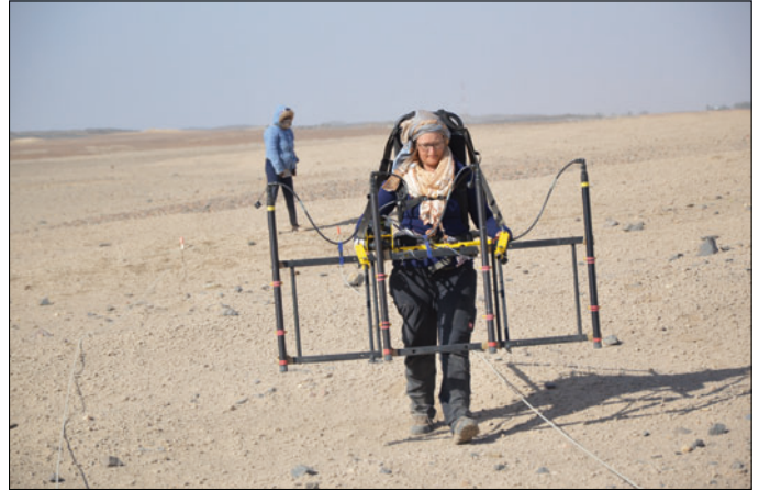
Plate 8. Magnetic prospecting of GiE 002 with the handheld Ferret 4.032 magnetometer in a quadro-sensor configuration (photo: G. D'Ercole).
