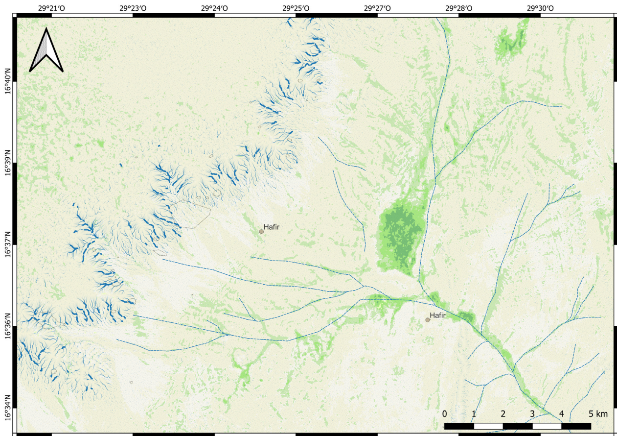
Figure 5. Hafirs , vegetation cover, and groundwater aquifers at the southwestern pediment of Jebel Nagashush. Vegetation cover classified using NVDI based on ESA Copernicus program Sentinel 2 A MSI multispectral data (stack T35QQU_20190827T082609). Groundwater aquifer mapping based on ESA Copernicus program Sentinel 1 B radar data (radargram s1b-iw-grd-vh-20200605t035555-20200605t035620-021893-0298d0-002). For map symbols, cf. Figure 3.
