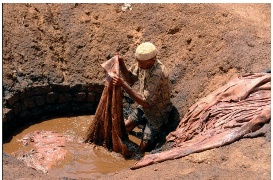
Colour Plate LI. Almyaelik tannery. A tanning pit, garrad seed pods can be seen floating on the surface (photo Elmonter Dafalla).
