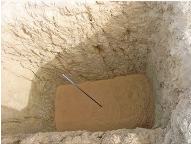
Plate 12. Goleid Plains, south west of Dongola. Sand trap of the type used to collect sand on the Goleid Plains and in the Wadi el-Khoni. The original pit is enlarged and a steel measuring rod inserted inside to assess volume change (photo R. N. Munro, March 2005).
