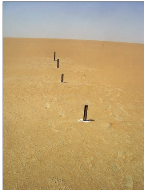
Plate 11. Baja. Array of vertical sand traps established by H. Abuzeid to measure sand drift (photo R. N. Munro October, 2004).
