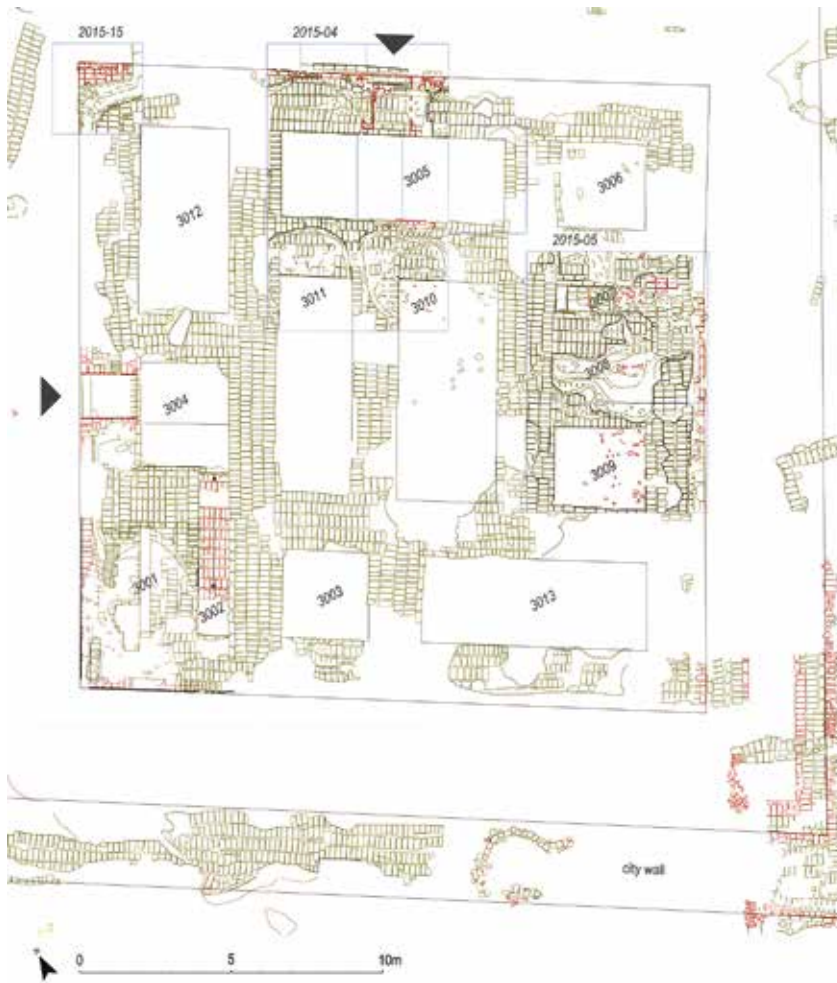
Figure 3. Plan of house H 3000 - black arrows mark the doorways; green: mud bricks; red: red bricks; blue: trenches of the 2015 season; scale 1:250 (drawn by C. Hof, 2015).
