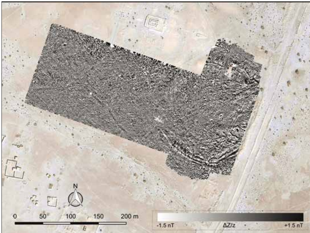
Figure 11. Magnetometry plot of the hafir in the Wadi Hadjala next to the 'Sun Temple' M 250 (Magnetic data by Eastern Atlas/Berlin 2015 (System: LEA-MAX; Registration: LEA-02; Sensor: 10 × Foerster FEREX 4031/4032 CON400/650); background satellite image: DigitalGlobe, acqu. date: 2.12.2010 (UTM Zone 36Q, WGS1984, source: GoogleEarth).
