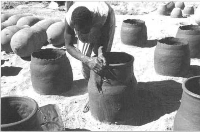
Plate 7. Kareima – Finishing with a wet cloth.
