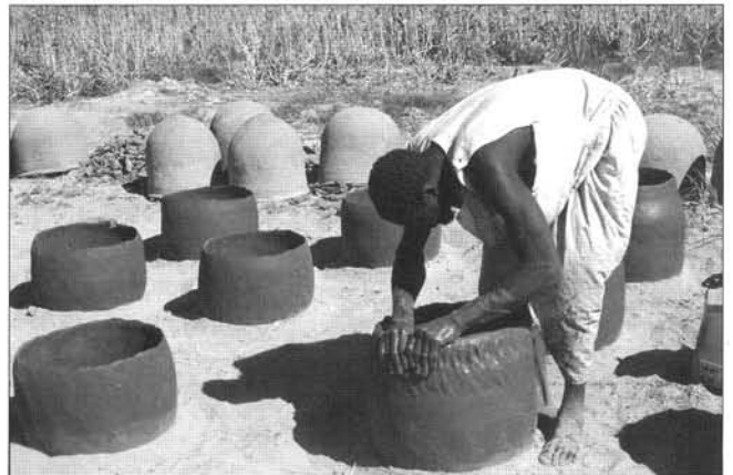
Plate 5. Kareima – Flattening the walls of the vessel.
