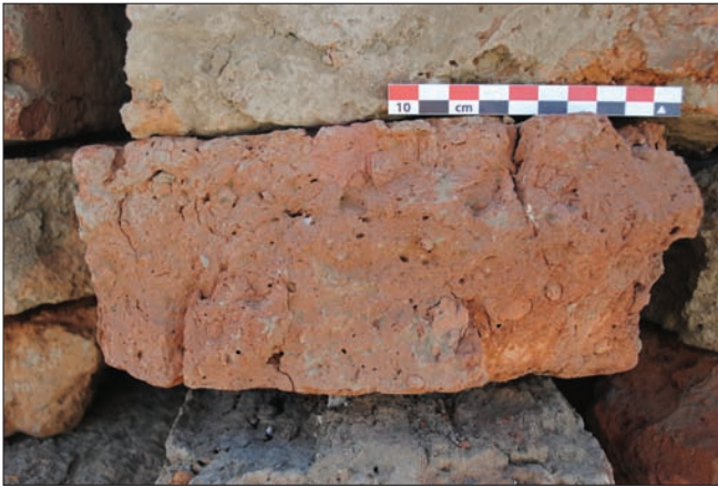
Plate 17. Broken red brick with inclusions of pot sherds.
